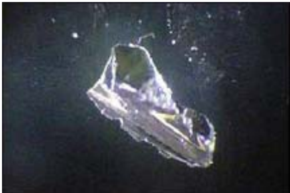
Adhesion chip – Warranty (Can occur from a manufacturing issue such as adhesion of molding to the glass surface along the glass edge.)
