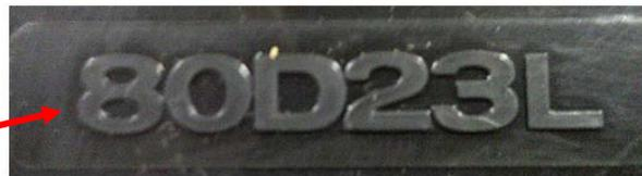
A JIS battery has the number embossed in the plastic on the top of the battery.
