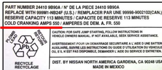
A CCA battery has the number displayed on the label attached to the top of the battery.
