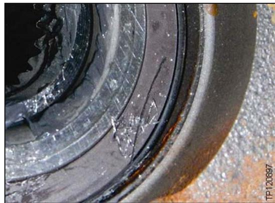
**NOTE:** Contamination on wheel speed sensor tone ring can cause intermittent errors.
