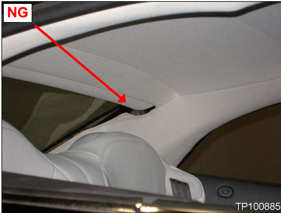
Wire rod improperly installed; headlining sags
